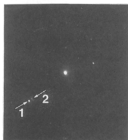
Figure 5 Dark-field image using the simultaneous z -beam condition shown in the inset with: 1g = [\bar{3}030]_{\text{Al}_2\text{O}_3} ; 2g = [220]_{\text{MgO}} .
